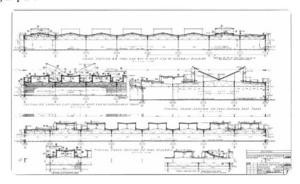
"Structural steel elements were prefabricated in New York by McClintic-Marshall Products (Bethlehem Steel Corp), shipped in a knock-down state to Stalingrad, via Black Sea and Volga, then assembled under the supervision of American builders and engineers selected by Kahn's firm"
